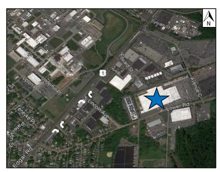
function as right-in/right-out only intersection with US Route 1/US Route 9. Therefore, vehicles leaving the site that plan to travel southbound on US Route 1/US Route 9 should be routed to one of the signalized intersections as illustrated in the figure to the right.
